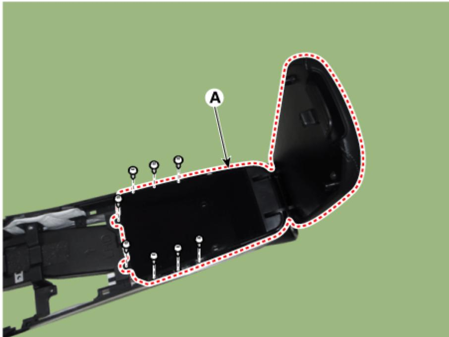
4. Remove the console armrest(A) after loosening the mounting screws.
